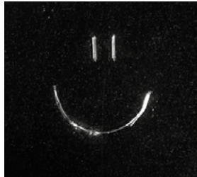
Scratch on acrylic glass – dark field backlight
