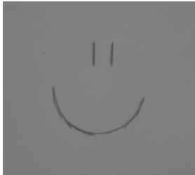
Scratch on acrylic glass – diffuse backlight
