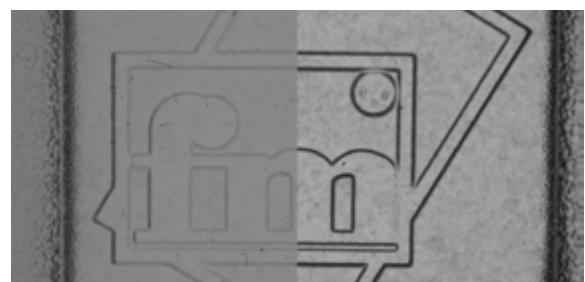
Transparent plastic with embossing – diffuse backlight
