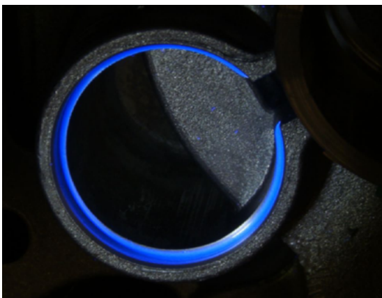
Cast part with fluorescent application under UV irradiation Left: fluorescence can easily be seen by the human eye
