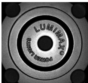
Conventional image capture using LED ring lighting
