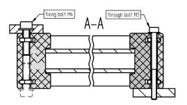
lateral installation using a size 5 sliding block in the circumferential nut
