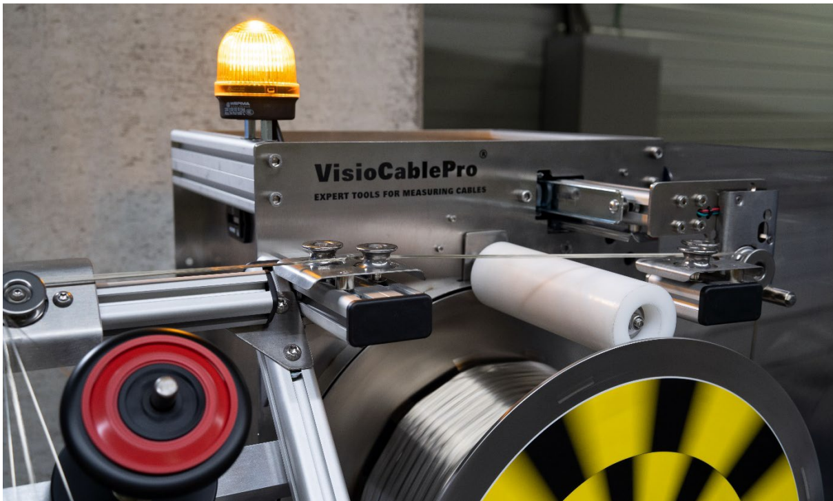
The ABU24 in an operational state – wire guided from the braiding spools via the distributor to the reel
