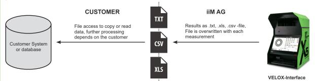
Scenario 2: The customer uses an existing database and wants to connect the VCPX5 to send testplans, logistical data, inspection features to select the article direct on the VCPX5. After the measurement, the results are sent back to the customers database. If the customer uses a CAQ system it is possible to analyse the results (charts, developments).
